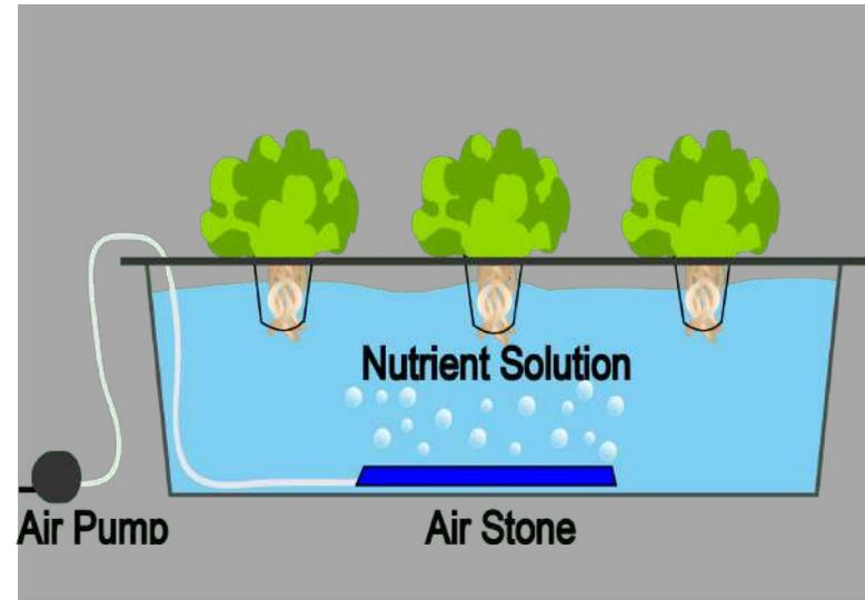
*visual representation of a single hydroponic system*
