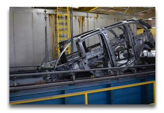
into the electrocoat tank for reuse. This "closedloop" process allows for process efficiency, cost savings and water and energy conservation. In order to maximize all the benefits of a closed-loop system, a high permeate flow rate is necessary.
